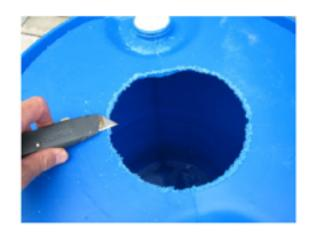
Tip: Use the sheet rock knife to remove all plastic burs, leaving a clean surface. It is especially important for the spigot hole because the shavings can get in the epoxy and leave room for a leak.
