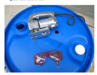
Cut the gutter inlet by first drilling a starter hole (drill in the piece that will be discarded) then use the ligsaw to cut out the inlet.
